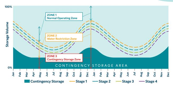
Figure 2 Illustration of water restriction curve zones.
