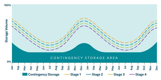
Figure 1 Example water restriction rule curve.
