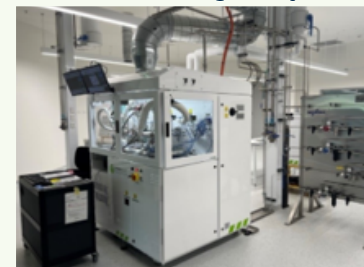
Hycel's G400 fuel cell test station
