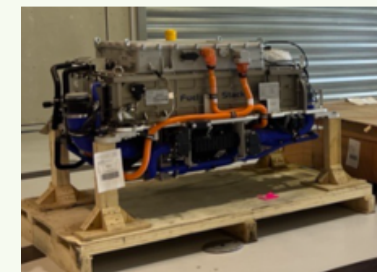
Hycel's 110kW fuel cell (pre-commissioning)
