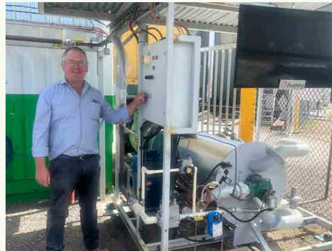
Austeng's Lead Engineer with the demonstration burner switching to run on a gas/H2 blend.
