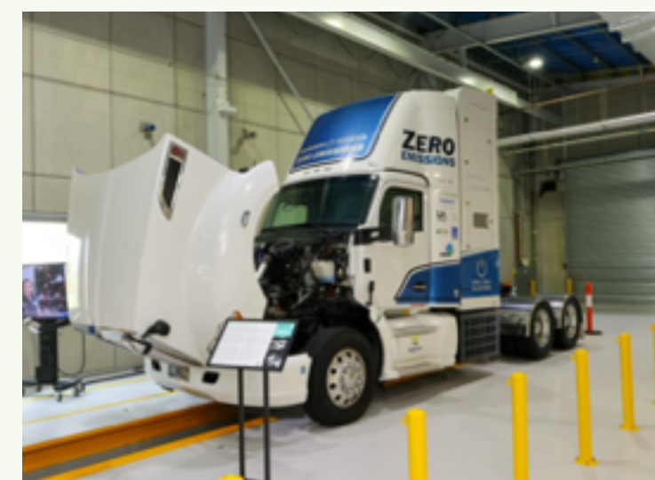
Kenworth T680 fuel cell prime mover in Hycel's Technology Integration Bay
